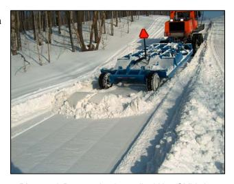
Photo 4.3 Remove back up piles! Use SMV sign.
