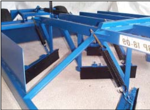
Photo 2.7 Beveled cutting blades
