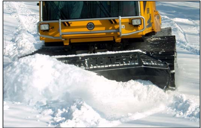
Photo 2.29 Typical front blade at work
