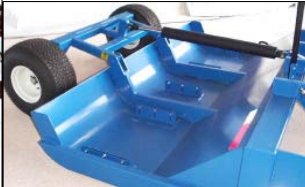
Photo 2.12 Radius lip on rear of pan
