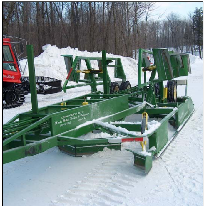
Photo 2.2 Drag with hydraulic wings
