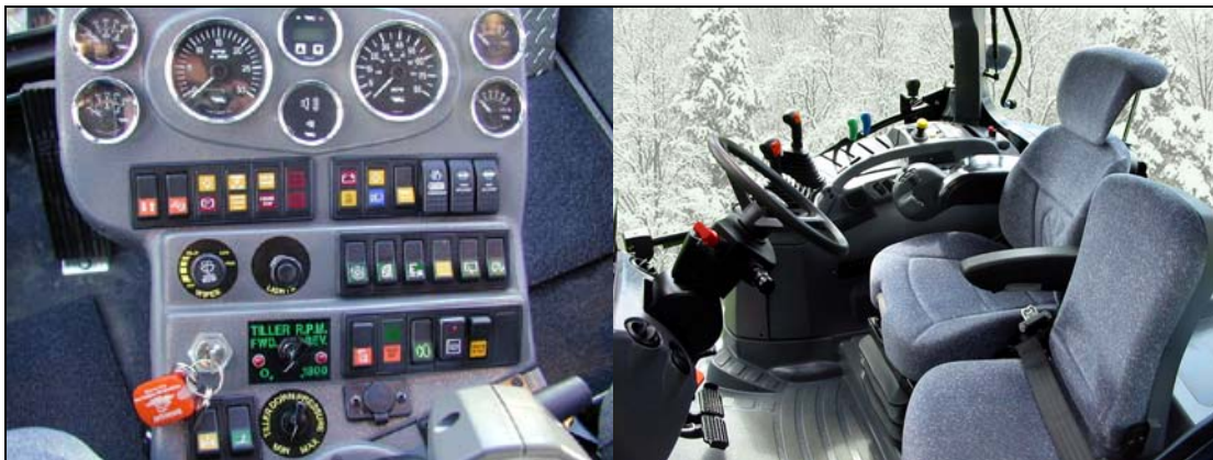
Photo 2.28 Typical controls in a tractor's cab
