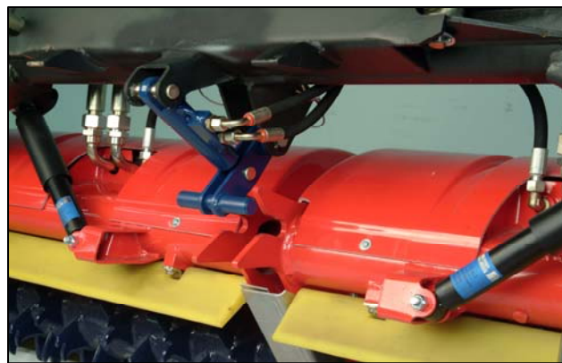
Photo 2.23 Flex tiller lockout device
