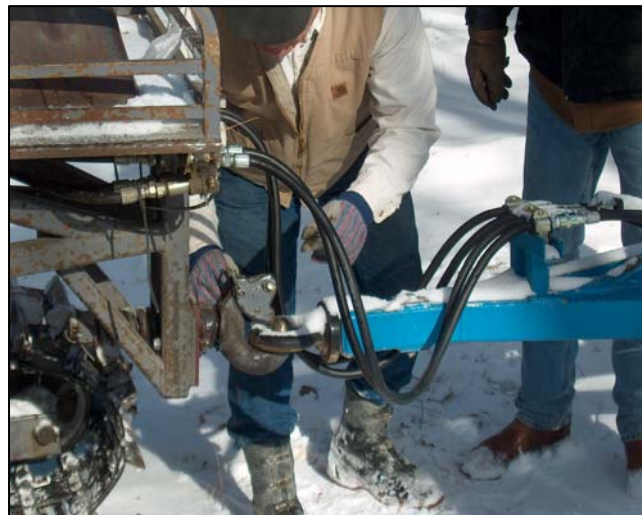
Photo 2.17 Quick-release couplings and shear pin in tongue of pintle hitch
