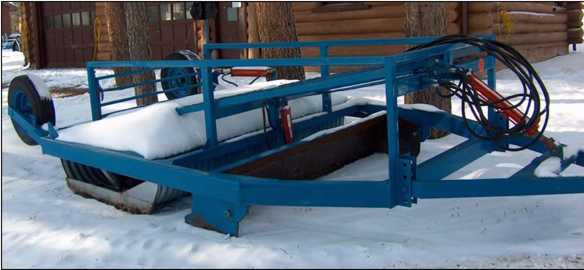
Photo 2.18 Typical single blade drag
