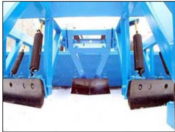
Photo 2.5 Spring tripping blades
