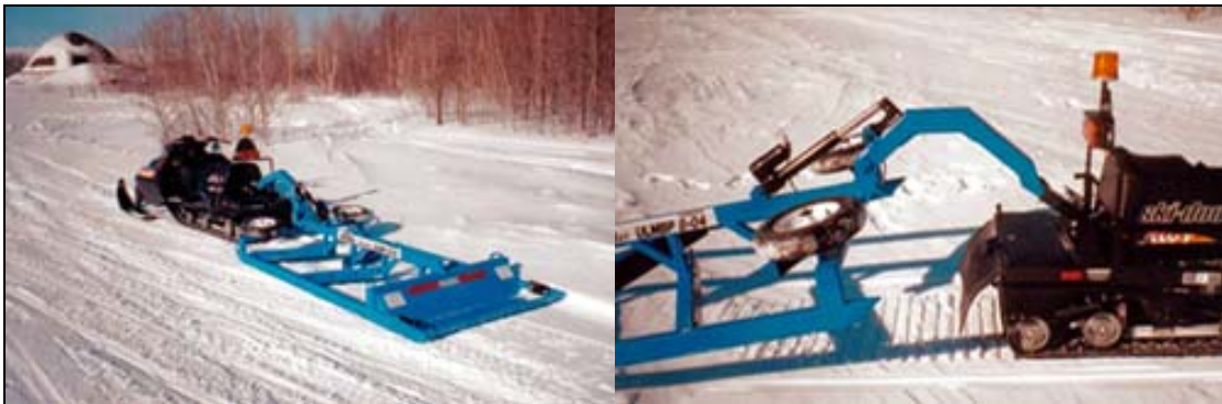
Photo 2.31 Typical snowmobile powered grooming unit
