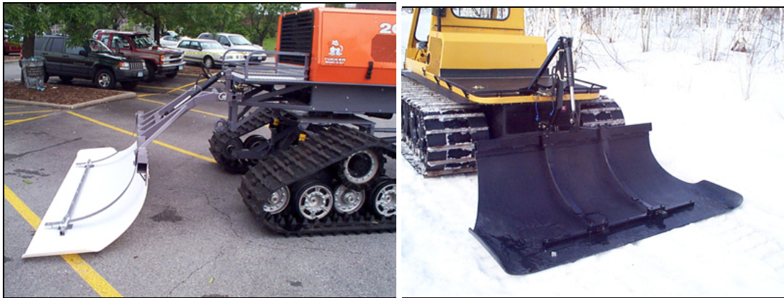
Photo 2.24 Typical compactor bars
