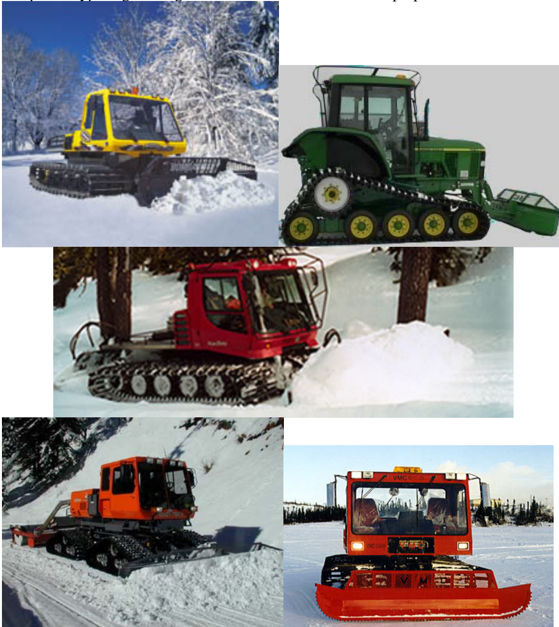
Photo 2.25 Typical grooming tractors
